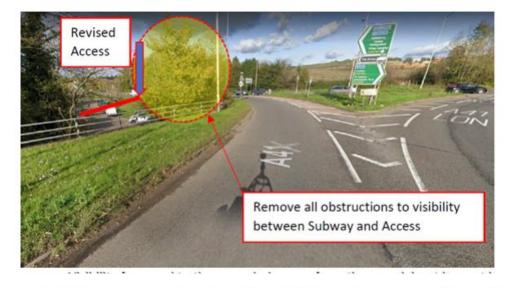
Visibility from and to the amended access from the roundabout has not been maximised. The parapet for the subway under the A41 is the only practical limitation on improving this. **The roundabout is within a 50mph speed limit, reducing to 40 mph on the exit into the A41, so DMRB visibility does apply especially as this route is a primary distributor.** In notes provided by the applicant it is suggested that Manual for Streets is appropriate. The Highway Authority does not concur with this point.
